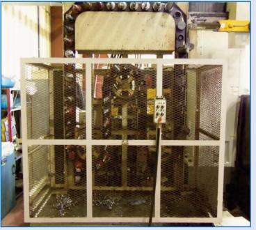
**NOMURA** FBA-70T CNC Table-Type Horizontal Boring Mill, 4.3" Spindle, Fanuc 16M Control, Travels: X-78", Y-51", Z-34", W-15.8", Rotary Table Size 55.5" x 63", Facing Head, 60 ATC
