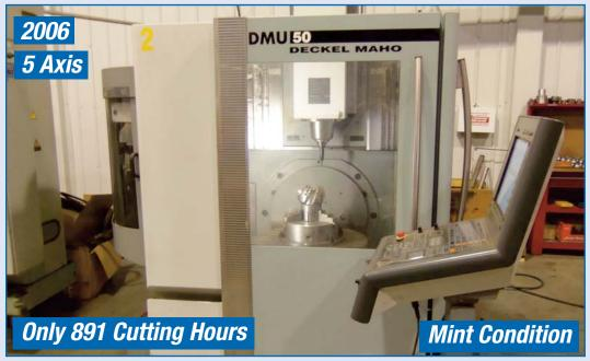
2006 **DMG** DMU 50, 5 Axis Universal, Hiedenhain iTNC30 3D Control Technology, Travels: X-19.6", Y-17.7", Z-15.7", Rapid Feed 39 FPM, Max 10,000 RPM, Cat 40, 16 ATC, Rotary Table Size 24.8" x 19.6", Only 891 Cutting Hours, sn 11415550874 (Note: DMG is under power and located offsite 10 minutes away.)
