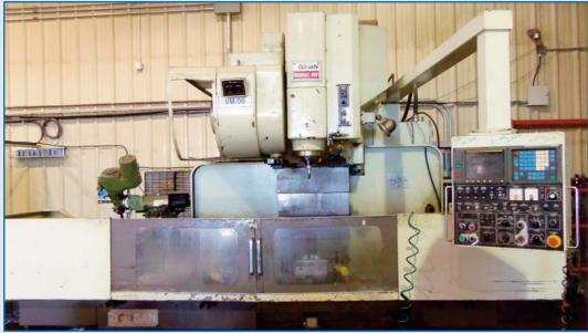
**DOOSAN** Doomac 80VR, Fanuc OM Control, Travels: X-78.7", Y-32.3", Z-23.6, 3,500 RPM, Cat 50, 30 ATC, sn MVC 055
